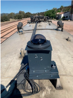
▲ A fish-eye camera on a train roof during a trial
