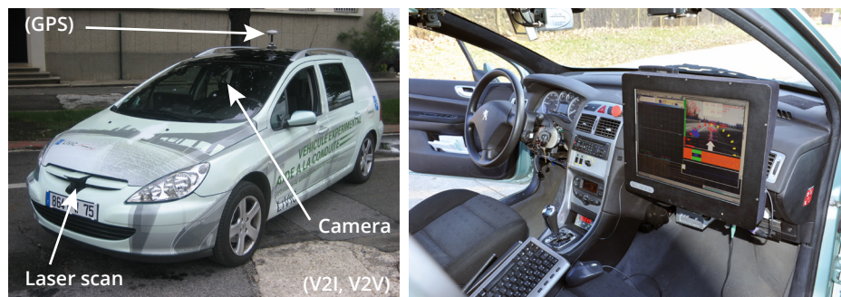
▲ CARLLA: the Ifsttar prototype dedicated to driving automation (ABV, Have-it, eFuture, and other projects)
