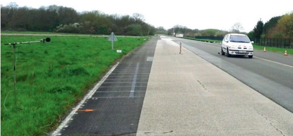
▲ Continuous measurement of embedded system rolling noise.
