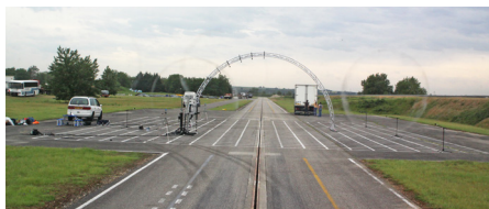
◀ GEODE project - acoustic emission measure of a vehicle
