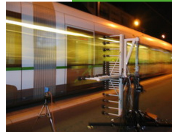
▲ Localization and characterization of tram noise sources through a microphone antenna
