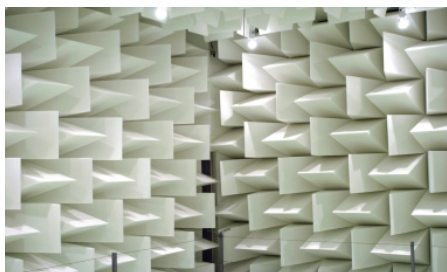
▲ Room semi-anechoic "Marin Mersenne" (SSA): insulated chamber whose walls and ceiling are padded to absorb the incident sound energy.
